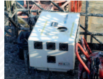
Figure 3 – Windcube LiDAR installed on the Schooner gas platform
